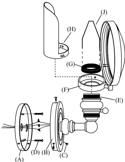
1. Remove back plate (A) from the base of lighting fixture (B) by unscrewing base screws (C) in counterclockwise direction.
