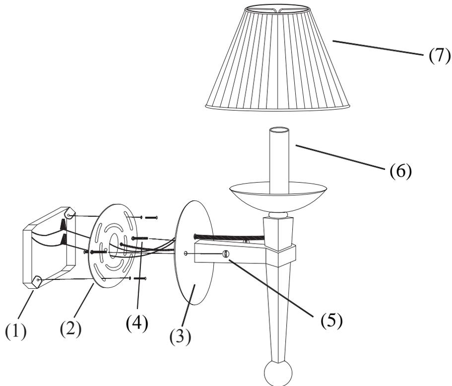
1. To detach the mounting plate (2) and the rod (4) from the light fixture, screw off the decorative screw (5) in counter-clockwise direction.
